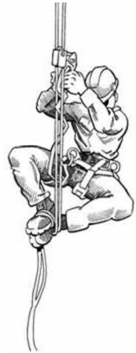
Paired ascenders secure the climber to the rope while footlocking.
